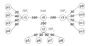
**Figure 4.** Network topology graph. Nodes represent *peers* (p) or *routers* (r) —among different *links* (the arcs). Arc weights correspond to link's *bandwidths*.
