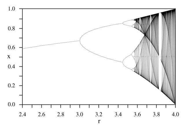
Figure 1: Bifurcations diagram of the logistic map (1), the vertical axis corresponds to the x value of the attractor and the horizontal axis corresponds the parameter  $\alpha$  (although it says r in the picture).
