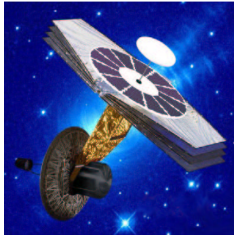
Figure 2.19: A SAFIR concept based on the segmented-mirror technology to be employed for the JWST (link). The telescope (in the lower left) would be composed of several mirror segments. Multiple layers of shielding would block the sun's heat and allow the cryocoolers to keep the telescope at a temperature of 4 K ( http://safir.jpl.nasa.gov ).
