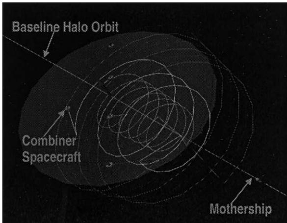
Fig. 1. TPF Interferometer Formation just after Deployment from the Mothership, spiraling around the Baseline Halo Orbit in a 100 m diameter 20-sided polygon (orange). The red arrow points at the star being observed.
