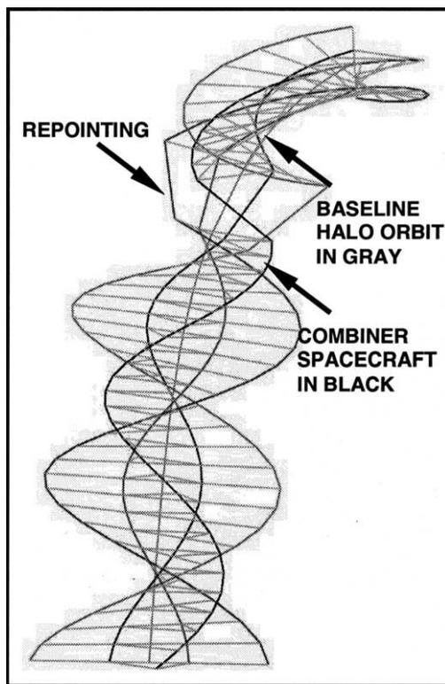
Fig. 3. Blowup of the small rectangle region in Fig. 2 for a close-up view of the formation. The colors of the curves are associated to different Spacecraft specified in the caption for Fig. 2. Note the re-pointing of the formation is shown by the linear portion of the curves.
