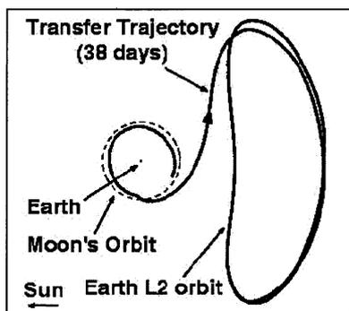
Fig. 6. The transfer from Earth–Moon  $L_1$  halo orbit (the near circular solid arc inside the lunar orbit) to a Sun–Earth  $L_2$  halo orbit in Sun–Earth rotating frame.
