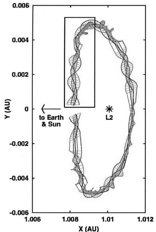
Fig. 2. TPF formation exaggerated to a 100,000 km diameter around the Baseline Halo Orbit. The horizontal yellow lines indicate the relative positions of the Baseline Halo Orbit (gray curve), the Combiner Spacecraft (black curve) and the four Collector Spacecraft (multicolor) at a particular time step.
